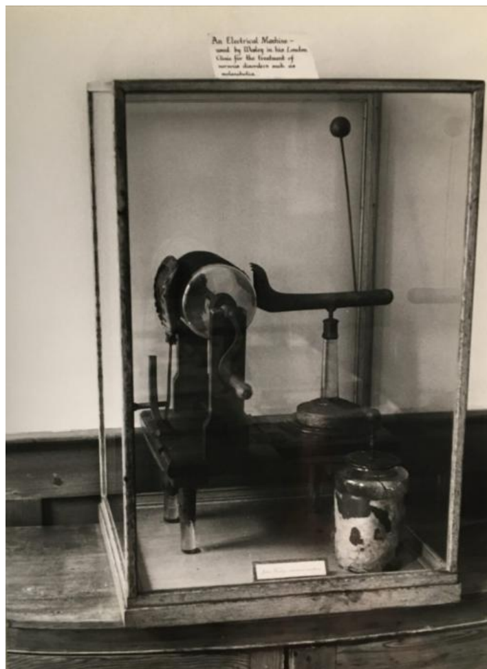
Figure 2. John Wesley's Electrical Machine. The crank to rotate and charge the glass sphere is visible. This was used by Wesley at his London home for the treatment of nervous disorders. Reproduced with the permission of the Trustees of Wesley's Chapel, City Road'.
